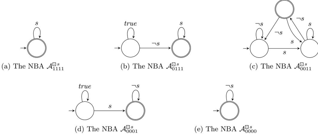
Fig. 1: The Büchi automata  $\mathcal{A}_\beta^{\square s}$  constructed in Step 1 of our monitor construction
