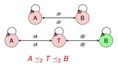
Definition of  $s \leq t$ : For every  $s \xrightarrow{i} s'$  there exists  $t \xrightarrow{i} t'$  s.t.  $s' \leq t'$   $\Theta^{1}$ : (truck)  $\Theta^{2}$ : (package)  $A \xrightarrow{i} A \xrightarrow{i} T \xrightarrow{iB} B$
