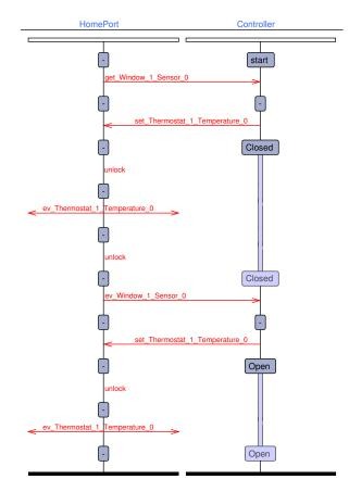
Fig. 5. Trace of an Execution of the Temperature Controller
