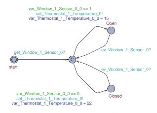
Fig. 4. Temperature Controller
