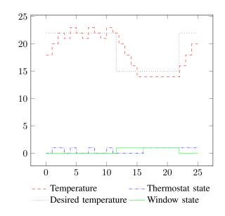
Fig. 9. Simulation of the control system
