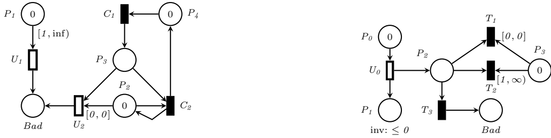
(a) A TAPG where Bad \leq 0 can be guaranteed by the controller under the continuous-time semantics (by exploiting Zeno behaviour) but not under the discrete-time semantics.
