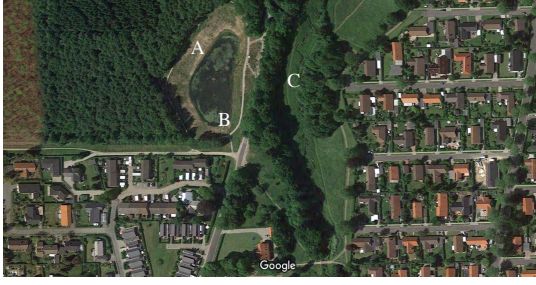
Fig. 1. Satellite image of the Vilhelmsborg Skov pond south of Aarhus, Denmark. A is the detention pond, where the outlet is located at B. Storm water is discharged in the stream labeled with C, which runs from the south to the north. Image from Google Maps.
