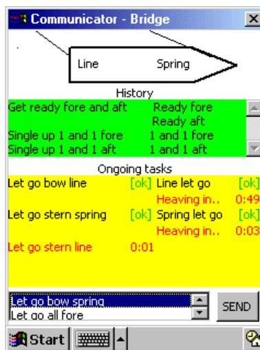
Fig. 7. The interface on the bridge
