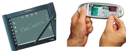
Figure 3. Direct pointers on handheld computers
