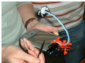
Figure 8. Wireless micro camera mounted on mobile device
