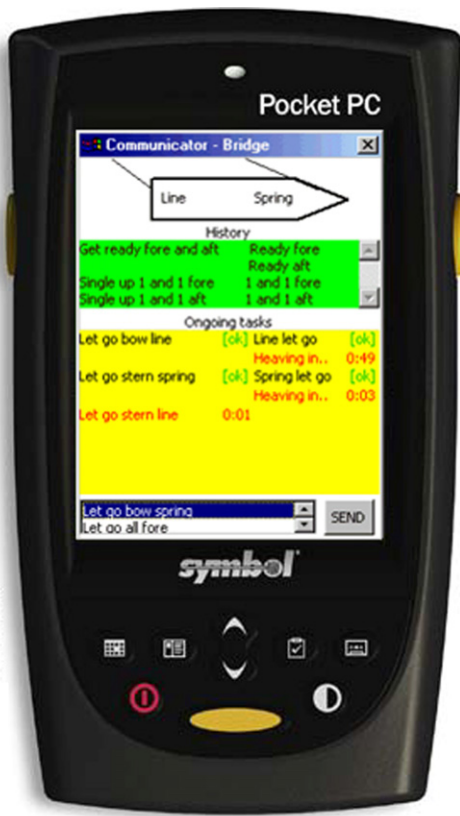
Fig. 17. The Maritime Communicator on a Symbol PPT8000.
