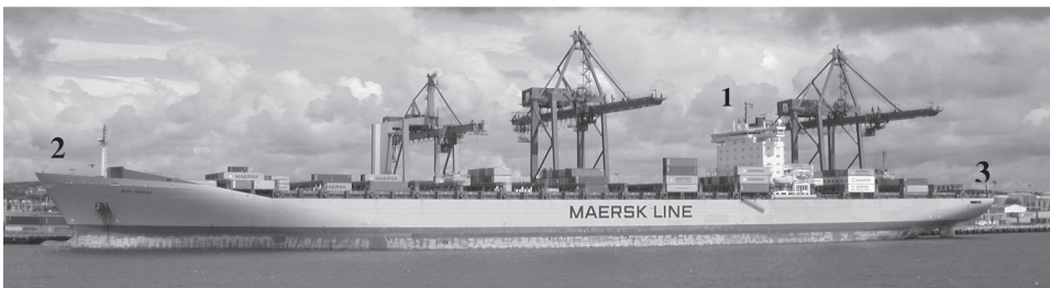
FIGURE 4 Sine Maersk in Gothenburg container terminal. 1 = bridge, 2 = fore area, 3 = aft area.
