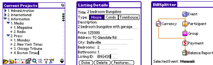
Figure 4. Menu selection, form filling and direct manipulation in graphical interfaces for the PalmPilot
