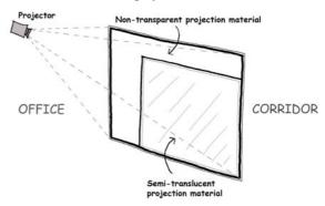
Figure 3. FrostWall projection onto a combination of opaque and semi-translucent projection material
