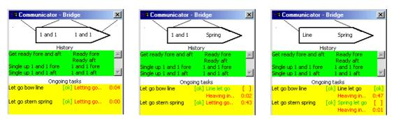
Fig. 11. Sequence of the visual representation reflecting the status of mooring
