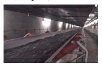
Figure 4. Underground conveyer belt transporting coal.
