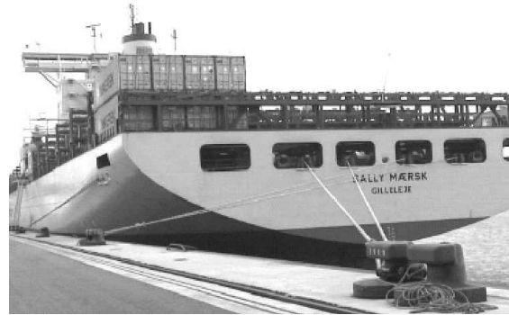
Figure 2. Sally Maersk with stern mooring lines
