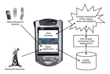
Figure 3. Just-for-Us prototype system architecture
