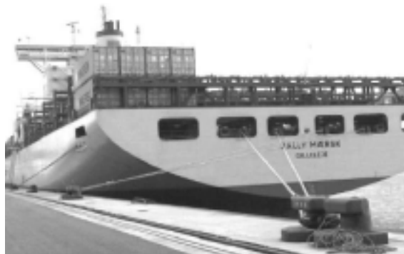
Figure 3: The aft mooring of Sally Maersk.
