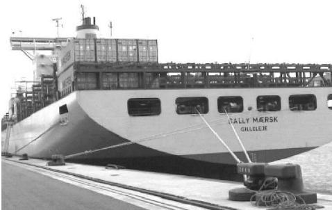
Figure 3: The aft mooring lines of Sally Maersk
