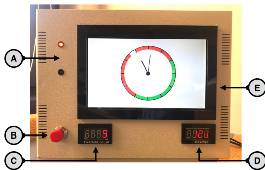
Figure 1. The Box: a) current electricity status, b) override button, c) override button presses, d) savings account, and e) 12 hour colour-coded clock.
