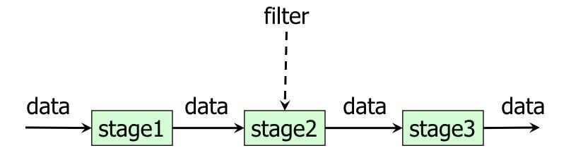
TBB: One stream of data – linear pipeline.
