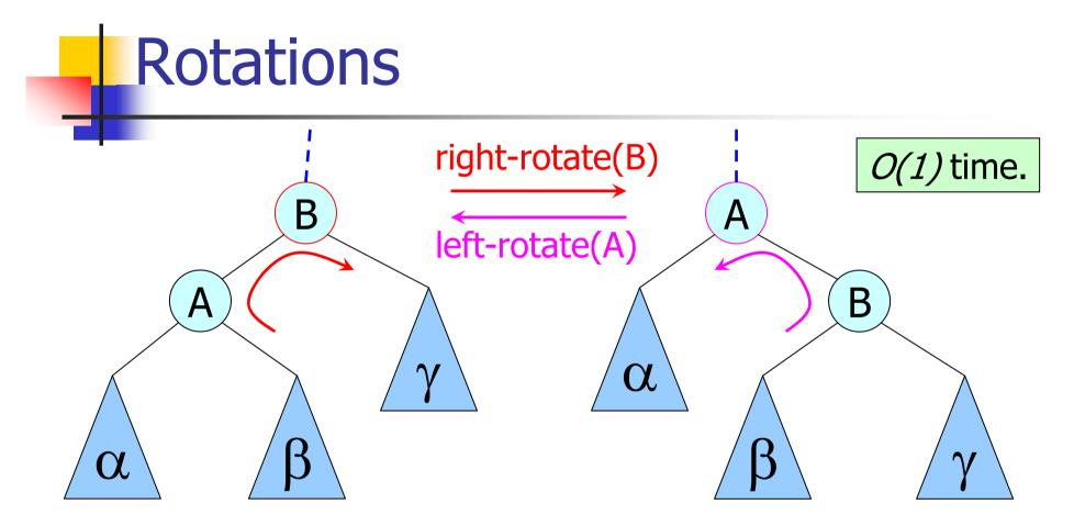
Important property: rotations maintain the in-order ordering of keys  $\Rightarrow$  binary search tree property maintained.  $\forall a \in \alpha, \forall b \in \beta, \forall c \in \gamma : a \leq A \leq b \leq B \leq c$ 14-11-06
