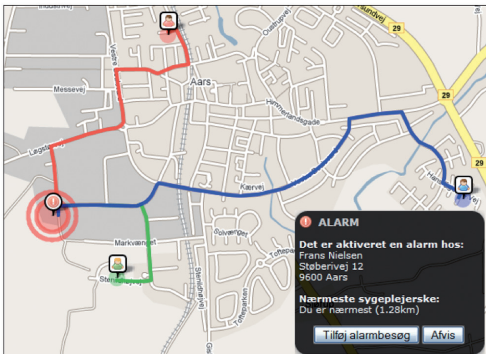
Figure 6. Patient alarm appearing as a pop-up message on the closest healthcare worker's screen along with information about location of the two most nearby colleagues.
