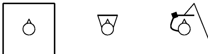
Figure 3: Full immersive displays for virtual reality: six-sided caves, hmds and booms (hmd mounted on stand and operated by hand)
